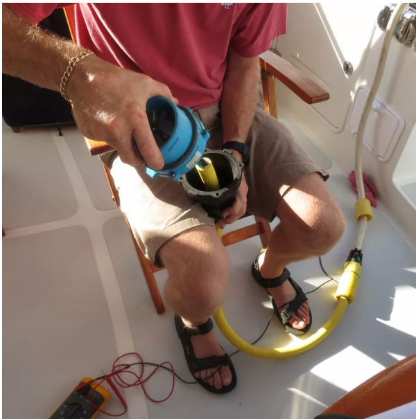
James wires a custom shore-power connection.
