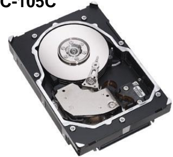
Hard Drives: 7W- 25W Temp Spec: 50C-60C
