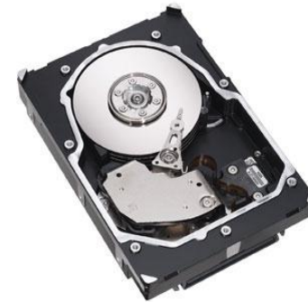
Hard Drives: 7W- 25W Temp Spec: 50C-60C
