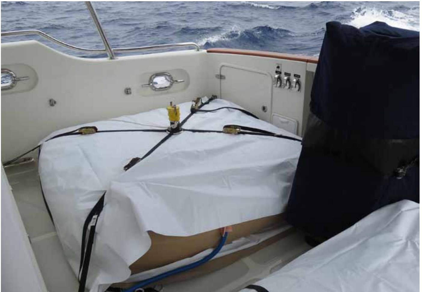
Above: The fuel bladder placement likely exacerbated the water ingress through the cockpit locker. Left: We expected winds in the 20-knot range, but instead were seeing steady 30-35 knots with gusts to 47.
