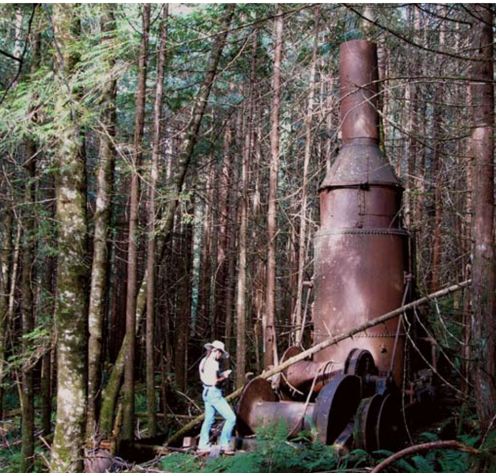
A massive steam donkey on a wooden sled stands in the railway corridor to Huaskin Lake.
