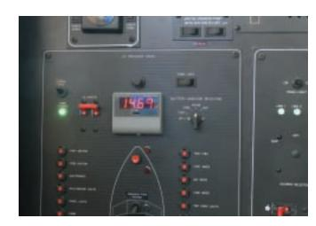
Many inverter control systems support a discharge floor to ensure that the discharge level doesn't fall below the minimum you select. We choose not to use this feature and have instead permanently mounted a large digital voltmeter where it is visible throughout the saloon. We can monitor charge level at a glance.
