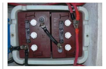
Battery bank design is made slightly more complex with golf cart batteries, since they are 6-volt batteries and most boats use 12-volt house battery banks. Here, the Trojan batteries are well secured in a battery box inside the boat's engine room, though the lid has been removed for this picture. It's important to have the battery box well ventilated for flooded lead acid batteries.
